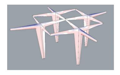
After plugging the model into karmaba, we found that the cantilever beams were subjected to the most stress. The intersecting beams at the center of the model were the least stressed area. We found that the beams facing inward were supporting each other through pinned connections. In terms of the cut outs (from prior iterations) we analyzed that only a small portion within the structure could be cut out, therefore forgoing the design aspect.
