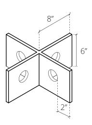
Pin connection connecting all 4 beams at center.
