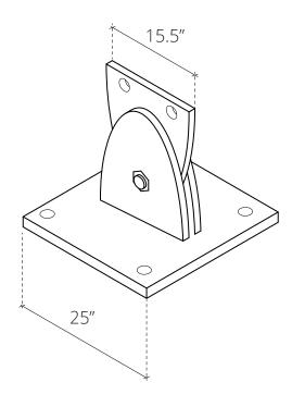
Pin connection connecting columns to steel plate. The Steel plate is anchored to the concrete foundation.
