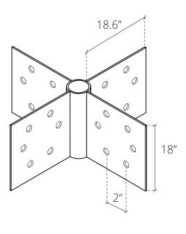
6 Holes are used to create a fixed connection between columns and beams.
